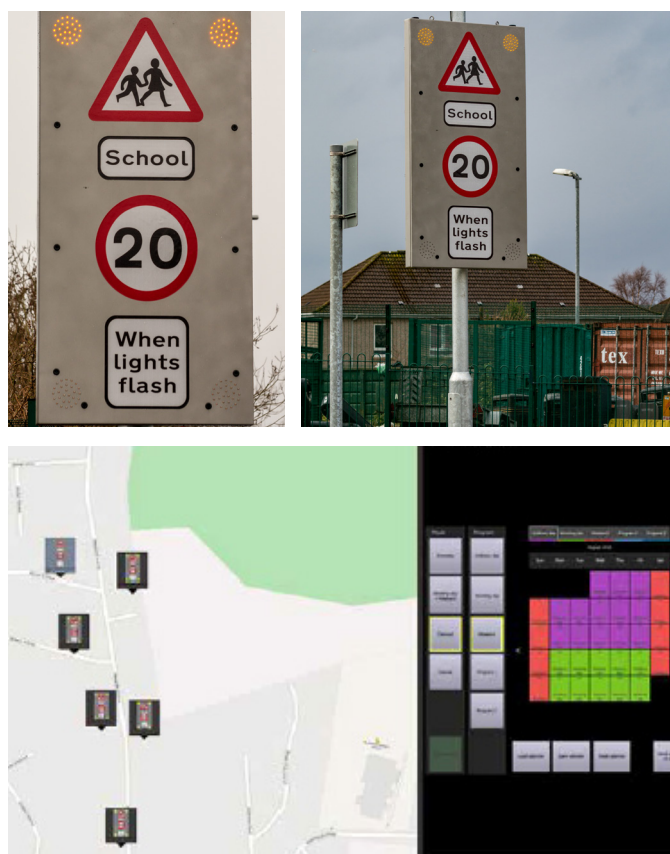
Left to right clockwise: Sign in action; Tablet control as well Cloud Control platforms
